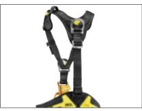
ASTRO BOD FAST full-body harnesses are equipped with a dorsal attachment point for attaching a fall-arrest system. In the event of a fall on this attachment point, a shorter adjustment of the length between the waistbelt and the leg loops means the load is taken up on the leg loops, allowing the user to remain suspended longer while awaiting rescue.
