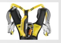
The harnesses have a stowage system for the MGO connectors on fall-arrest lanyards on each shoulder strap. In the event of a fall, the system releases the MGO connectors and allows the absorber to be deployed.
