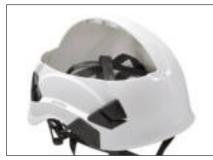
VERTEX helmets have a six-point webbing suspension system, conforming to the shape of the head for maximum comfort. Shock absorption is achieved through deformation of the external shell.
