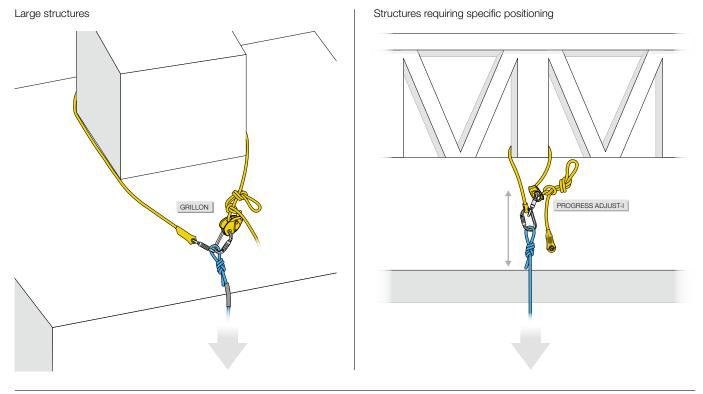
Temporary anchors with multiple configurations.
