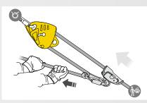
The integrated progress-capture pulley with very large diameter sheave mounted on sealed ball bearings rotates in only one direction for excellent hauling efficiency. The lower connection point can be used to create different types of haul systems.
