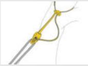
The system enables multiple setup configurations on the branch: wrap-around or choked. It has an adjuster that allows precise length adjustment of the friction saver.
