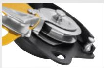
The faceted sheave creates additional friction zones for the rope and thus provides extra braking for lowering heavy loads.
