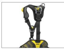
The AVAO BOD and AVAO BOD FAST full-body harnesses are equipped with a dorsal attachment point for connecting a fall-arrest system. In the event of a fall on this attachment point, a shorter adjustment of the length between the waistbelt and the leg loops means the load is taken up on the leg loops, allowing the user to remain suspended longer while awaiting rescue.
