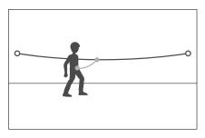
ABSORBICA-I single lanyards are designed especially for protection on a horizontal lifeline or on an elevated platform.
