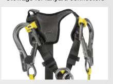
The harnesses have a stowage system for fall-arrest lanyard connectors on each shoulder strap. In the event of a fall, the system releases the MGO connector and allows the absorber to be deployed.
