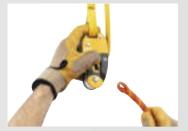
Rope installation is possible only if the friction saver is correctly set up, and the gated attachment point is locked.
