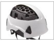
The liner of STRATO helmets is designed in two parts: EPP (expanded polypropylene) and EPS (expanded polystyrene), for reduced weight. Shock absorption is achieved through deformation of the liner.
