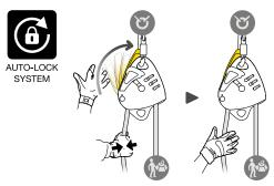
Hauling is possible at any time, without manipulating the handle.
